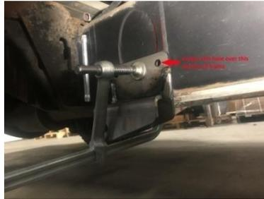
11. Use a 1/2" Drill bit to mark the center location of the hole. Next use a 3/8" drill bit to drill a pilot hole through the frame. Once the pilot hole is drilled all the way through then use the 1/2" Drill to open the hole up.
