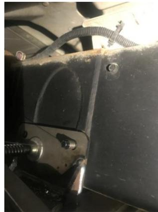
15. Install the washer over the pull wire and use it to help hold the bolt in place while removing the pull wire. With the pull wire removed install the lock nut onto the bolt. Use an 8mm socket to hold the bolt while tightening the nut with a  $\frac{3}{4}$ " wrench. Make sure the 8mm socket stays fully engaged on the bolt to prevent stripping the hex.
