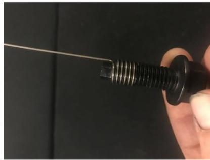
14. Feed the wire through the hole drilled in the back side of the frame rail and gently pull the wire and bolt through the hole drilled for the bracket.
