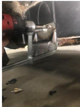
12. Now on the inside of the frame rail in the oval section where the frame is the thinnest, drill a 3/8" pilot hole and then open it up with a step bit until the head of the bolt fits through the hole (about 1 1/8")
