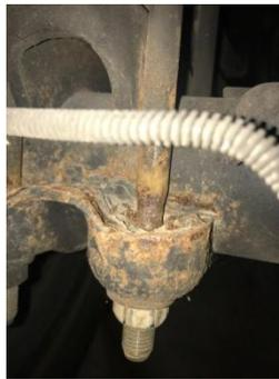
4. Remove the nuts from the U-bolts. It is recommended to do one side at a time to avoid the axle from shifting. With the nuts removed slide the lower plate off the U-bolts.
