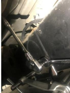
16. With the bolt tightened to ensure the bracket doesn't move drill the remaining three holes and repeat the same procedure on the other side.
