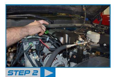
Remove the Resonator from the turbo mouthpiece.
