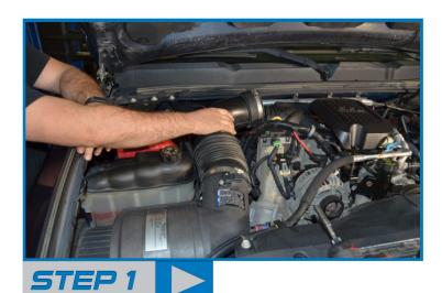
Loosen the worm gear clamp securing the intake tube to the turbo mouthpiece.
