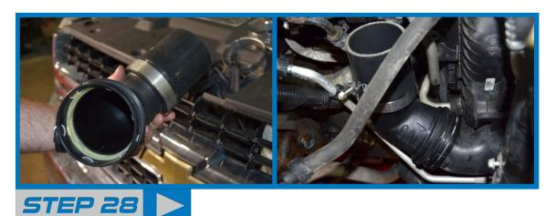
Remove the plastic elbow from the factory cold side tube. The end that you will need is labeled CAC. It is recommended to clean the elbow up with engine degreaser and warm water. Install the supplied 3" boot and clamp on the elbow. Reinstall the metal wire clip on to the elbow and slide it onto the intercooler making sure it locks into place.
