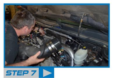
Using pliers release the clamp holding the PCV hose assembly to the turbo mouthpiece. Loosen the V-band worm gear clamp holding he mouthpiece to the turbo and remove.
