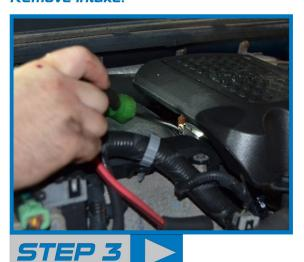
Remove resonator box from intake mouth piece. Use a flat head screw driver and loosen the worm gear clamp.
