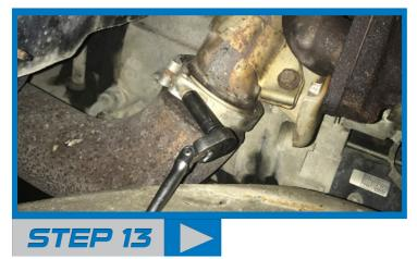
Connect the down pipe to the front pipe using the factory V-band clamp.
