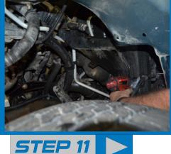
Remove the intake box support bracket form the core support.
