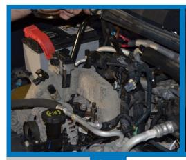
Tuck the wiring behind the cold side Using a plastic clip removing tool to get it out of the way.
