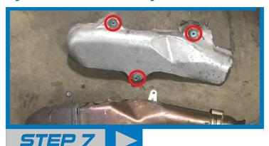
The heat shield on the down pipe must also be removed. This is held in place with (3) 10mm bolts.
