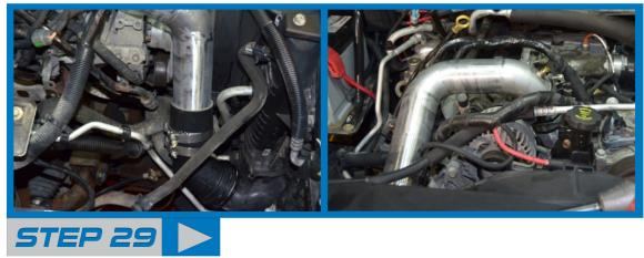
Slide the 3" boot and clamp onto the bridge neck. Next install the new cold side placing it into the boot at the intercooler first and then into the bridge neck.
