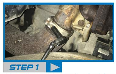
Using an 11mm socket remove the v-band clamp that holds the factory down pipe to the front pipe. With the nut removed use a flat head screw driver to release the v-band.
