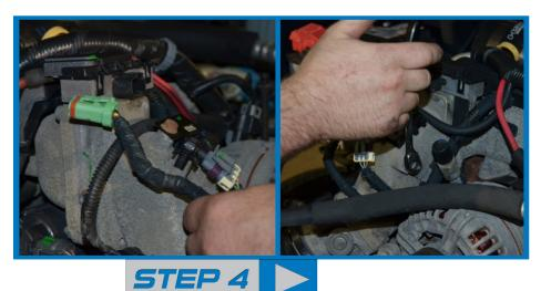
Unplug the grid heater, MAP sensor, and throttle valve from the factory cold side. Remove the 10mm bolt securing the harness to the side of the cold side.
