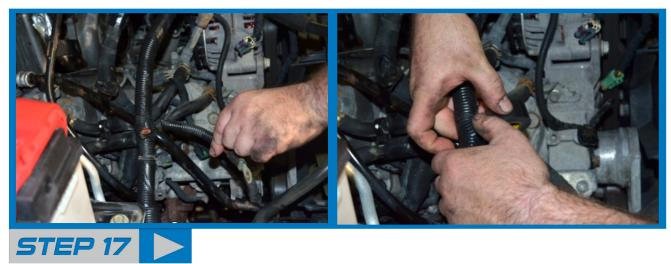
There is also a power wire that needs to be eliminated that went to the grid heater. Cut the end of the cable off and wrap the end of the wire with electrical tape or heat shrink and tuck it into the harness and tape it closed.
