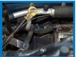
Install routing it from the heater core to the steel bypass tube that comes up behind the turbocharger.
