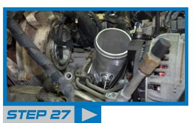
Reinstall the steel fuel lines and reconnect them to the rubber lines. Make sure to reinstall the hose clamps.
