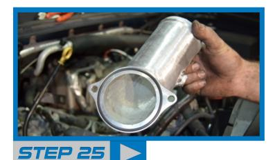
Install the new bridge neck on to the bridge using the supplied studs and 12 point 10mm nuts. Make sure the o-ring stays in place. With the nuts installed tighten them with a 10mm boxed end wrench.
