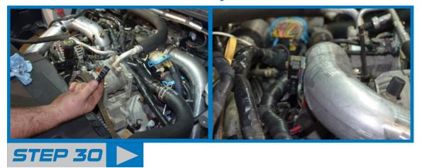
Install the MAP sensor in the new cold side using the original bracket and hardware.
