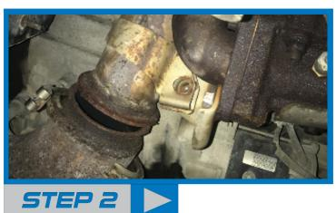
Remove the bolt holding the down pipe to the up pipe support plate using a 14mm socket.
