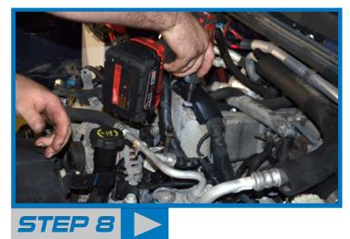
Remove the 4 T-30 torques screws holding the plastic wire loom form the top of the cold side.
