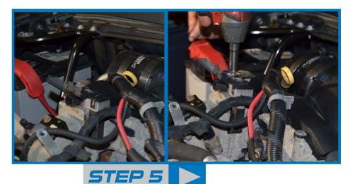
Open the cover on top of the grid heater and remove the 10mm nut securing the power wire.
